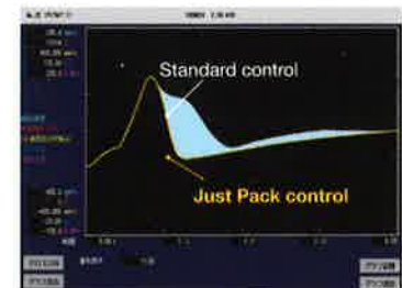
The graph above shows a comparison of differences in the holding process after completion of the first injection process using standard and Just Pack controls. It can be seen that the pressure range shown in the pale blue segment is surplus to needs
